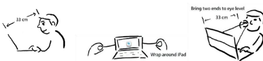
Figure 5. Setting the correct test distance without using a hood.
